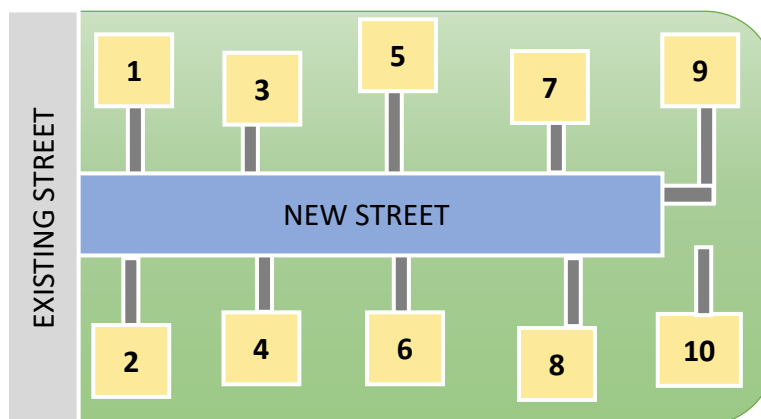
Figure 9 – Numbering along a side street
